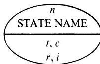
Fig. 13. CCITT Recommendation X.21 quiescent states. Each state is represented by an ellipse wherein the state name and number are indicated, together with the signals on the four interchange circuits that represent that state. Each state transition is represented by an arrow and the equipment responsible for the transition (DTE or DCE) is indicated beside that arrow. Here n is the state number, t is the signal on transmit interchange circuit, c is the signal on control interchange circuit, r is the signal on receive interchange circuit, i is the signal on indication interchange circuit; 0 means steady binary 0 condition, 1 means steady binary 1 condition, 01 means alternate binary 0 and binary 1 conditions, OFF means continuous OFF (binary 1) condition, ON means continuous ON (binary 0) condition, and X means any value.
